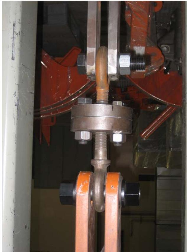
The test rack was designed so that it would attach to and hydraulically pull the plates apart. The purpose behind the test was to incrementally increase the amount of force used to pull on the plates up to the point where separation occurs between the plates. This would indicate the point at which the clamping force has been overcome and provides us with a way to verify what that clamping force actually is.
