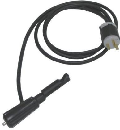
The T59521 Reverser Handle plugs into the reverser on the control stand. The other end (plug end) plugs into the electrical jog receptacle. A push button switch in the handle is depressed to jog the locomotive forward or backward using the locomotive battery and traction motor to provide power. The locomotive engine need not be started, eliminating smoke and noise.
